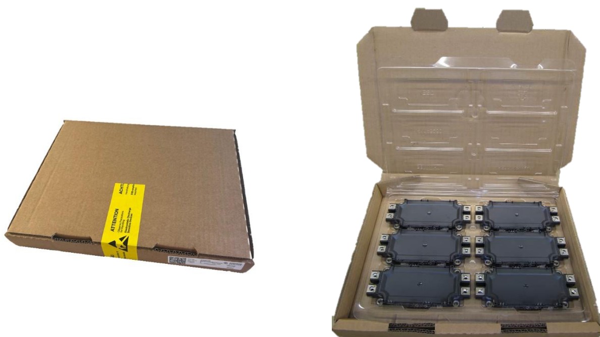
Figure 4: Cardboard box with modules in transparent ESD tray
